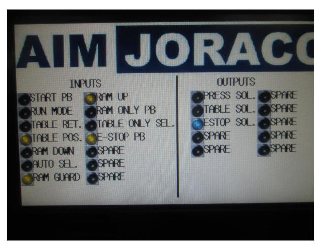
TABLE POS Should be Lit when index unit in station.
