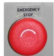
To Restore the System, the Off-Stop-Run switch must be set to Off, the Emergency Stop Button reset (twist) and/or the Ram Guard repositioned. Turning the Off-Stop-Run switch to Stop will restore the compressed air and the indexer is ready to run.
