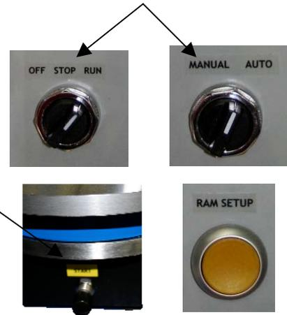
**Rotary Table Only** - Set Off-Stop-Run switch to STOP position and Manual-Auto switch to MANUAL. Set ROTARY TABLE ONLY toggle switch to the up position. Press the START button, the rotary table will index one position and stop, the ram will remain up. Press START to repeat.
