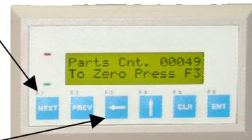
**Screen 2** - Batch Count screen is used to set the quantity in a batch. When the batch count is enabled and the parts count reaches this number, the indexer will stop (Auto Mode ONLY). The Parts count must be set to zero (see above) before continuing operation.
