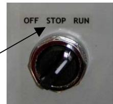
To set the batch count, the Off-Stop-Run switch must be in the Stop position. Press ENT then CLR, cursor should now be flashing. Press the Up arrow to increase the digit, Down arrow to decrease the digit. When correct digit is displayed, press left arrow to shift the digit to the left and repeat until the desired Batch Count is displayed. Press ENT again to set Batch count.
