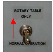
**Manual Mode** - Set Off-Stop-Run switch to RUN and Manual-Auto switch to MANUAL. Press the START button, the rotary table will index one position, the ram will descend and return. Pressing the START button will repeat the sequence.
