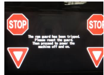
Photo 2.12 Resetting Ram Guard
