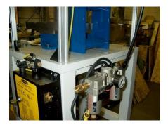
The Filter, Regulator Lubricator (FRL) is a component which cleans the air and lubricates the internal valving and seals, as well as providing adjustable pressure.
